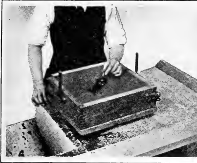
FIG. 504. PLACING PART TO BE RAMMED UP IN THE COPE.
